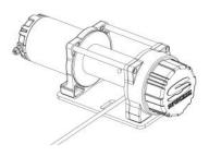
While looking at the hoist from the motor side, no matter how the feet are oriented, the drum must rotate clockwise to power in and counterclockwise to power out for the brake to function properly. Otherwise, the brake may work against the motor while lifting.
