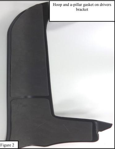
Locate the driver side upper A-pillar gasket, lower A-pillar gasket, and mounting bracket. Place both gaskets onto the mounting bracket as shown in Figure 2 and cut out the five holes on the lower A-pillar gasket to allow re-installment of the five bolts.
