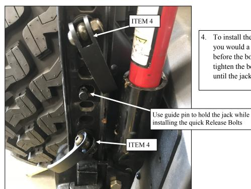
4. To install the Quick Release Bolts (4), thread them in as you would a normal screw but with the lever open. Just before the bolt gets tight, close the lever. Loosen or tighten the bolt as necessary by repeating this process until the jack feels secure.
