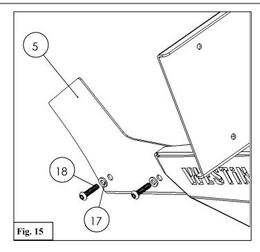
The quarter panel will be sandwiched between the hardware and the Closeout Panel (5).
