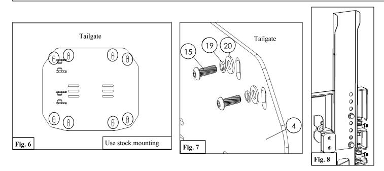
9. Install the Tire Mount (5) to the Tire Carrier (1) along with the CHMSL Light Relocator (10) using the supplied M12 Hardware. See Figures 8-10.
