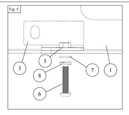
7. Align and tighten all hardware as specified: M8 to 18 ft-lbs, M10 to 35 ft-lbs.
