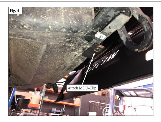
6. Loosely attach the skid plate to the bumper and brackets via the U-clips (2,3) with the supplied M8 hardware. See Figure 5.
