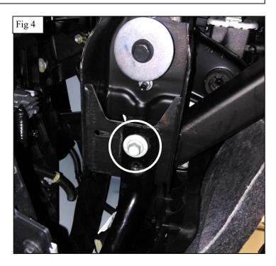
7. Locate the tray mounting brackets. Using supplied M12 hardware, loosely assemble the tray brackets by sliding into the frame. See Figure 5-8. Use the square washer on the inner sides of the frame rail.
