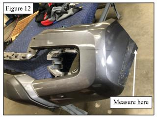
b. Using the ruler as a straightedge, draw a small line on the face of the bumper to the next edge. Using the ruler and line you just drew, measure 1 inch below the line. Mark dots at each edge. See **Figures 13 & 14** for reference.
