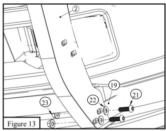
15. Align and adjust the grille guard and brackets as necessary and then torque all: M10 hardware to 30-35 ft-lbs, and M12 to 50-55 ft-lbs.
