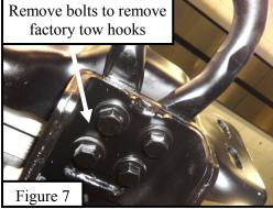
7. Starting on either side of the vehicle. Locate (1) Lower Mount Bracket (Item 2/3) and from the front of the vehicle install it where the tow hooks were. Align the bracket with the vehicle frame at the same location that the factory bracket was removed. Loosely install using (4) M12 hex head cap screws, (8) M12 hex nuts, (8) M12 split lock washers and (12) flat washers (Items 6 - 9). See Figures 11 and 12.
