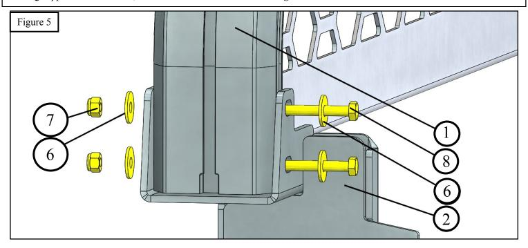
8. Once all components are positioned as desired. Tighten all M8 hardware to 15-18 ft-lbs and all M12 to 50-55 ft-lbs. Note: When tightening M8 hardware that was used to install hoop and screen assembly on step 7, push the top of the HLR rack towards the cab of the truck to maintain straight while tightening.
