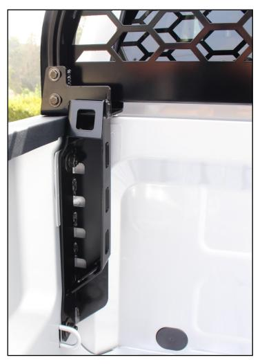
8. Once all components are positioned as desired. Tighten all M8 hardware to 15-18 ft-lbs and all M12 to 50-55 ft-lbs. Note: When tightening M8 hardware that was used to install hoop and screen assembly on step 7, push the top of the HLR rack towards the cab of the truck to maintain straight while tightening.
