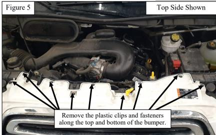
Remove the license plate and factory license plate holder. Remove the two bolts and carefully pull off the bumper assembly. See Figure 6 & 7 for reference. <u>Note:</u> Make sure any wiring connectors secured to the bumper are unplugged prior to removal.
