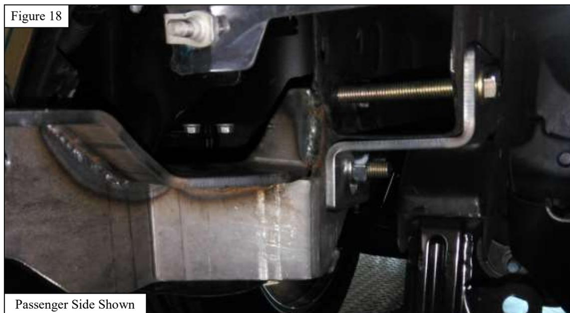
18. With help, loosely mount the Grille Guard Base to the previously installed mounting brackets using the supplied M10 and M12 hardware. See **Figure 19** for reference. *Note: Loosely install the upper strap hardware just to hold the grille guard center. This hardware will be used to install the HDX Wings in the next step.*
