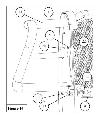
21. Adjust the Assembly as desired and tighten all hardware: M8 to 18 ft-lbs, M10 to 32 ft-lbs, M12 to 55 ft-lbs.
