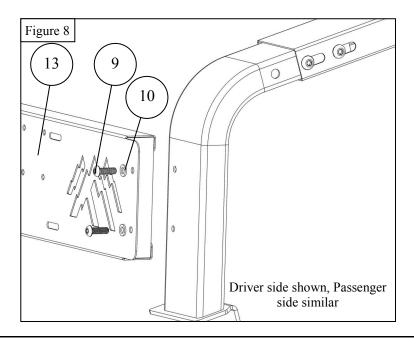
8. Using M8 hardware, mount the 2 top support brackets to the rack assembly. **Note: The top support bars can be aligned as needed for your application. See Figure 9**
