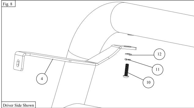
7. Adjust the bull bar as needed and torque all hardware as specified: 3/8" to 20 ft-lbs, M10 to 38 ft-lbs.
