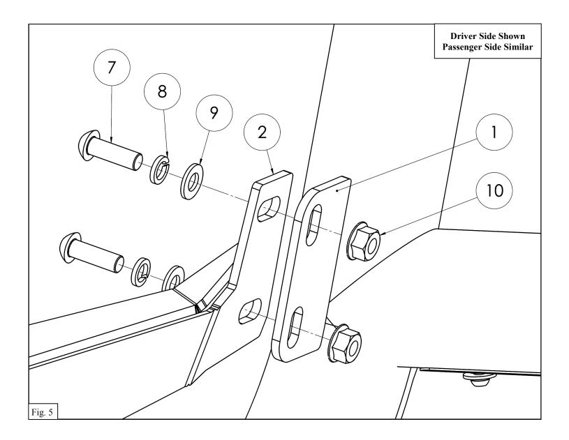
7. Adjust bull bar and brackets as necessary and torque all hardware according to the following specifications: M10 to 25-30 ft-lbs and M14 to 88 ft-lbs.
