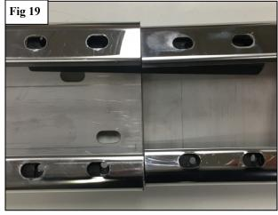
13. Place the supplied step pad into the holes to connect the two Step Bar sections (1 & 2). Place the supplied thread cutting nut on each of the plastic stems. See Figures 20 and 21.
