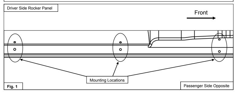
Loosely secure (1) Front Mount Bracket (item 3) to the rocker panel using the supplied M10 hardware . See Figures 1 & 2.
