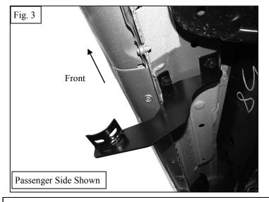
3. Locate the Center threaded mounting holes. Select (1) Center/Rear Mounting Bracket. Attach with (2) 10mm Hex Bolts, (2) 10mm Lock Washers and (2) 10mm Flat Washers. Do not tighten hardware at this time. **See Figures 4-6**
