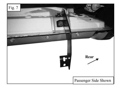
5. Attach Sidebar to the mounting brackets with (6) 10mm Bolts. Do not tighten hardware at this time. **See Figures 8-11.** *Note: Do not slide or rotate Sidebar on cradles, or damage to the finish may result.*
