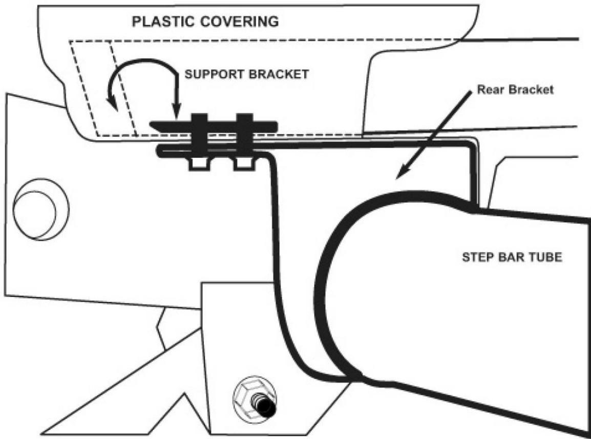
FIGURE 3 - REAR PASSENGER-SIDE BRACKET
