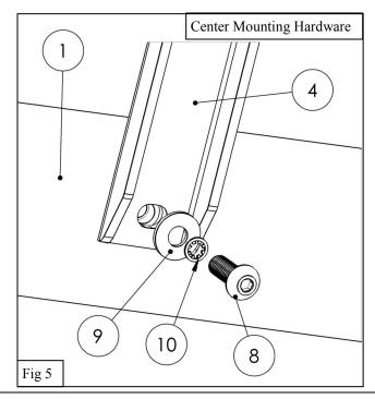
4. Adjust the installed step bar as desired and torque all hardware: 1/2" to 50-55 ft-lbs, M10 to 25-30 ft-lbs, and OE Body Mount Bolts to 120 ft-lbs.
