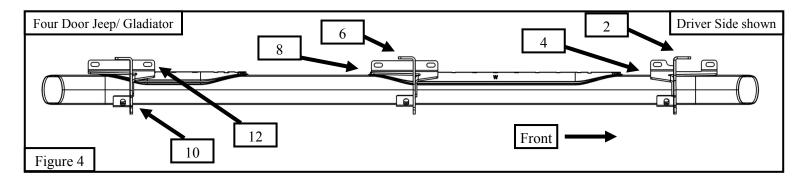
8. Align step bar and brackets to desired positioning then torque and tighten all: M8 hardware to 16 ft-lbs and M10 to 32 ft-lbs.
