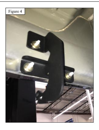
5. At the center passenger side mounting location, loosely install Mounting Bracket Base (3) with preassembled Passenger Center Mounting Bracket (Item 6) using the supplied M8 hardware. See **Figures 5 & 6** for reference.
