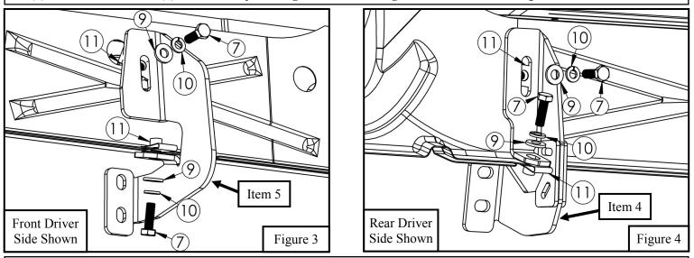
For Step Board installation, tilt board at an angle to insert brackets into mounting locations. With the previously installed mounting brackets use the supplied M8 hardware with the short M8 hex head bolt, then loosely install. See Figures 5 & 6.
