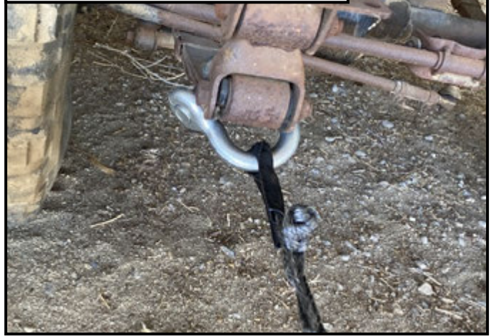
Figure 21b –Utilize a steel shackle when securing the winch line to sharp edges
