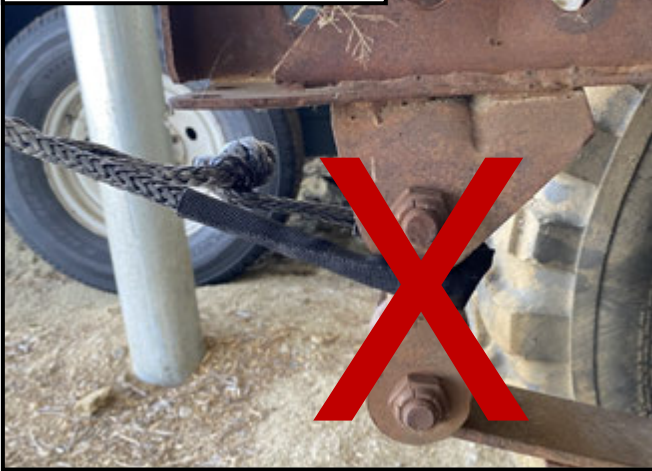
Figure 21a –Never attach the soft shackle to a sharp edge
