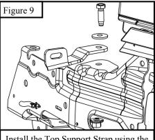
Install the Top Support Strap using the factory hardware attached to the mounting location. Driver Side Shown.
