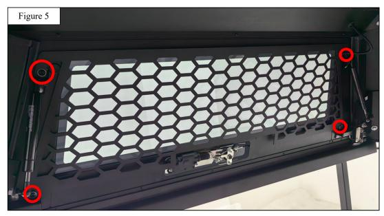
Adjust the Rear Door Mesh Protector to the appropriate position. Tighten all bolts M6 hardware to 5-7 ft-lbs and all M8 hardware to 15-18 ft-lbs.
