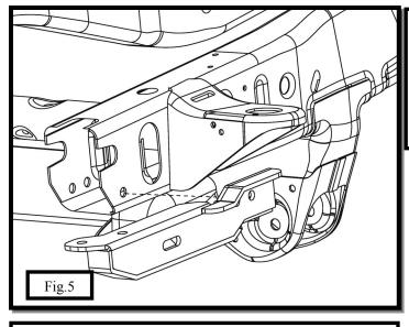
ONCE YOU MOUNT THE BRACKETS TO THE EXISTING HOLES, MARK THE HOLES THAT REQUIRE DRILLING TO PROPERLY MOUNT EACH BRACKET. **NOTE:** A **TRANSFER PUNCH IS SUGGESTED.**  TO PROPERLY INSTALL BRACKETS YOU MUST DRILL HOLES TO THE FRAME. IN ORDER TO DO SO YOU MUST ALIGN THE BRACKETS TO THE FRAME USING THE EX-SISTING MOUNTING HOLES. AS SHOWN ON (FIG. 5)
