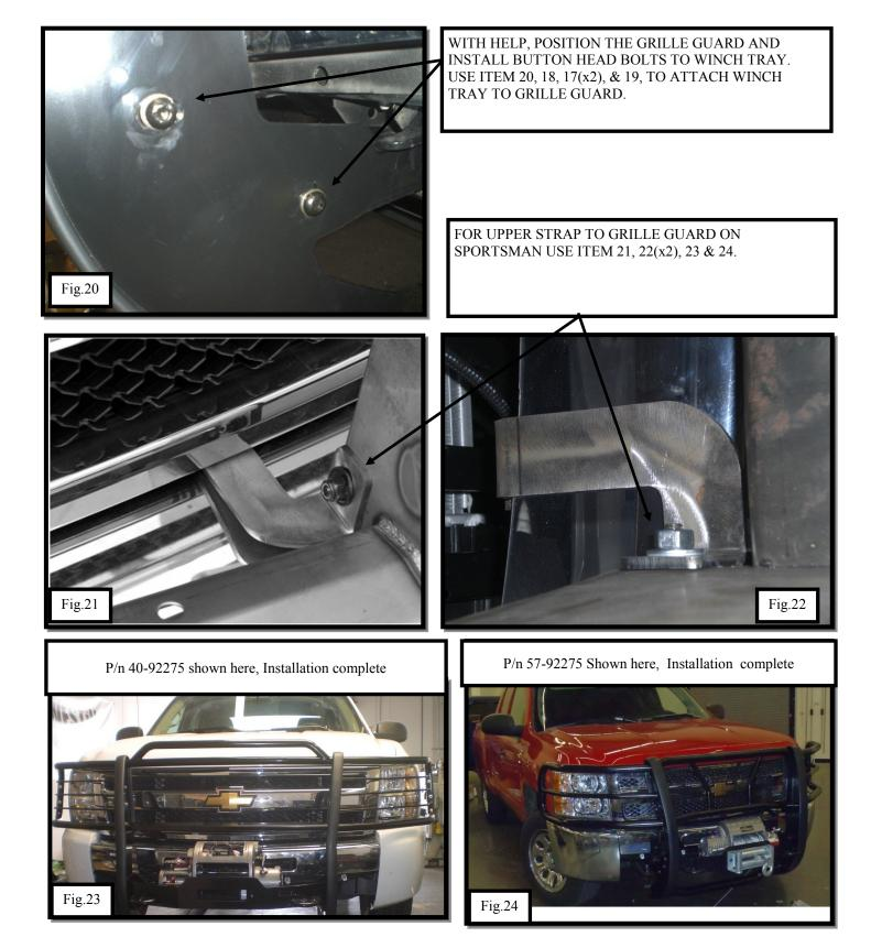
ALIGN & ADJUST GRILLE GUARD AS NECESSARY THEN TIGHTEN ALL REMAINING HARDWARE: M10 to 30-35 ft-lbs., M12 to 50-55 ft-lbs.
