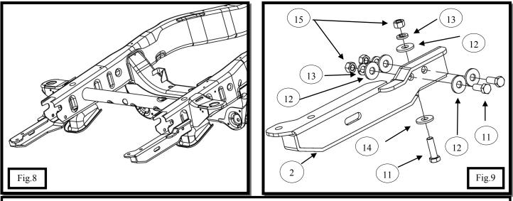
INSTALL THE DRIVER SIDE BRACKET TO THE FRAME USING (2) M12 HEX HEAD BOLTS, (4) M12 FLAT WASHERS, (2) M12 LOCK WASHERS, AND (2) M12 HEX NUTS. ON THE BOTTOM DRILLED HOLE, USE (1) M12 HEX HEAD BOLT, (1) M12 THICK FLAT WASHER, (1) M12 FLAT WASHER, (1) M12 LOCK WASHER, AND (1) M12 HEX NUT. *(REPEAT FOR PASSENGER SIDE MOUNT BRACKET).* **NOTE: DO NOT FULLY TIGHTEN AT THIS TIME.**
