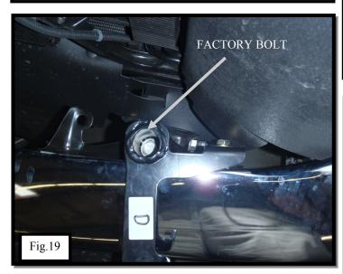
REMOVE THE TWO TOP EXISTING FRAME BOLTS ONE AT A TIME AND PLACE THE UPPER STRAP (ITEM 4 & 5) IN THAT LOCATION. DO NOT FULLY TIGHTEN AS YOU NEED TO ADJUST LATER. **NOTE: FOR HDX MOUNTING PLEASE REFER TO** (FIG.19 & 20)
