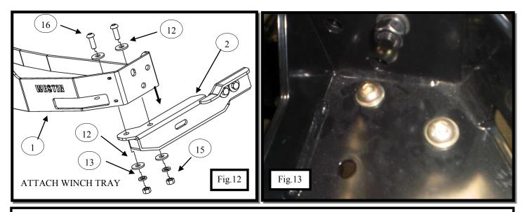
TO ATTACH WINCH TRAY USE (4) M12 BUTTON HEAD BOLTS, (8) M12 FLAT WASHERS, (4) M12 LOCK WASHERS, & (4) M12 HEX NUTS. YOU MAY NOW ALIGN AND ADJUST MOUNTING BRACKETS AND WINCH TRAY. NOTE: DO NOT FULLY TIGHTEN IF INSTALLING A GRILLE GUARD KIT. NOTE: TIGHTEN ALL FASTENERS IF NOT INSTALLING A GRILLE GUARD KIT INCLUDING MOUNTING BRACKETS. TORQUE ALL M12 FASTENERS TO 50-55 ft lbs.
