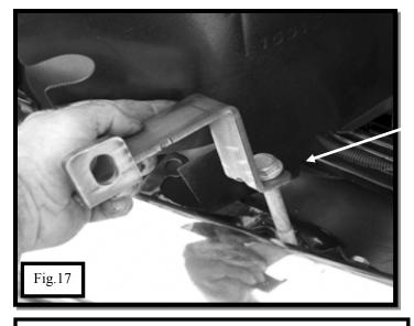
RE-INSTALL FACTORY GRILLE SHELL AT THIS TIME, LINE UP THE CLIPS AND GENTLY PUSH GRILLE SHELL INTO PLACE. DO NOT RE-INSTALL TOP COVERS.
